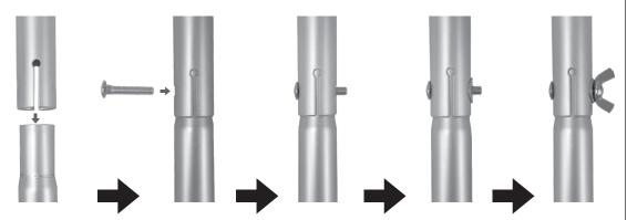
Repeat installation onto the other Curved Bar (B or C) with the other assembled Armrest (D) and Leg (E). Ensure the Wingnuts (H) are tight.
