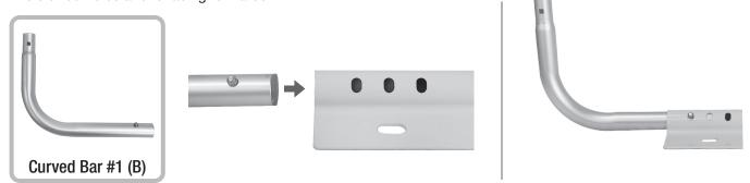
Repeat with Curved Bar #2 (C) and insert it into the other side of the Mounting Bracket (A).
